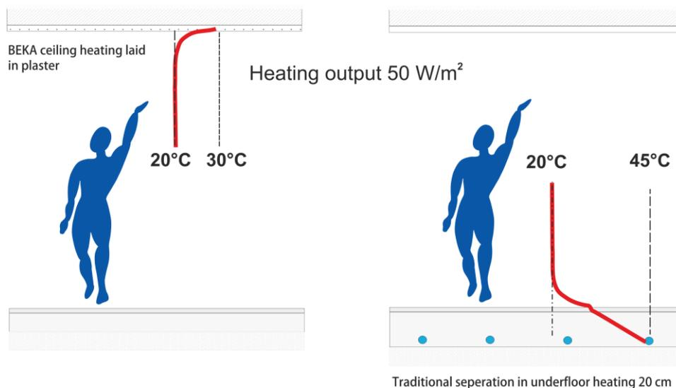
As a rule, with BEKA ceiling heating a supply temperature of around 30°C is sufficient to heat the room adequately. Traditional underfloor heating always requires 40°C or more, depending on the separation and the type of floor covering. BEKA ceiling heating "saves" on the supply temperature and therefore produces more efficient results when energy efficiency is compared with that of traditional underfloor heating.
