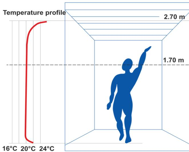
BEKA ceiling heating should preferably be integrated in thin layers in the ceiling construction. With plaster ceilings, this means that a layer of plaster only 15 mm thick is sufficient to cover the capillary tubes. But also any conventional suspended ceiling construction made of gypsum plasterboard or a metal cassette ceiling can be activated for ceiling heating without any problem.
